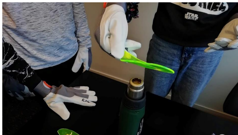
Figure 1: Students bending an acrylic rotor blade using a heat gun.
