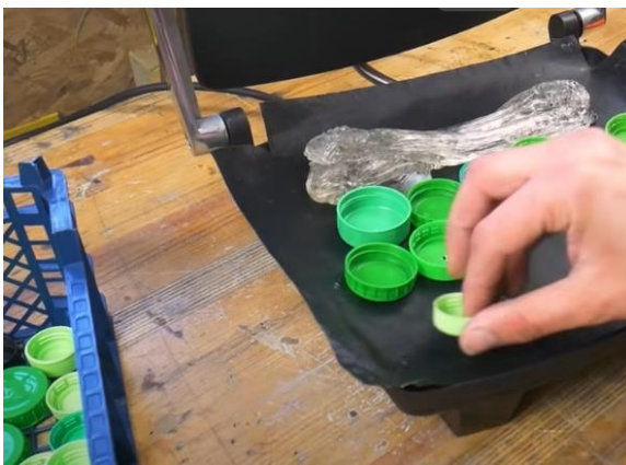
Figure 9: Plastic caps are heated and melted for recycling purposes
