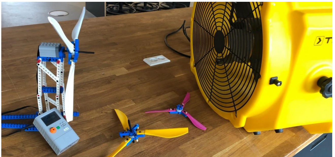
Figure 5: Example of wind turbine which is ready for testing with the wind machine. The turbine is connected to an energy-meter.
